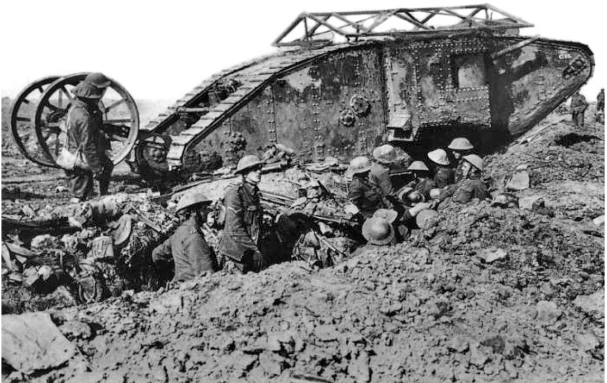
An early model British Mark I "male" tank, named C-15, near Thiepval, 25 September 1916. The tank is probably in reserve for the Battle of Thiepval Ridge which began on 26 September. The tank is fitted with the wire "grenade shield" and steering tail, both features discarded in the next models. Photo by Ernest Brooks.
